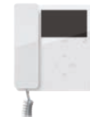
7548 Tab 4,3 - surface mounting video entryphone with handset, 4,3" LCD display, teleloop facility for hearing aids, white
